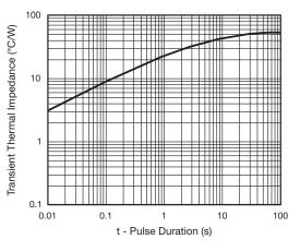
Fig. 7 - Typical Transient Thermal Impedance
