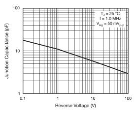
Fig. 6 - Typical Junction Capacitance
