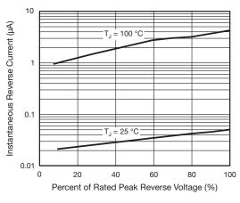
Fig. 5 - Typical Reverse Characteristics
