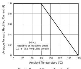
Fig. 1 - Forward Current Derating Curve
