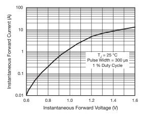
Fig. 4 - Typical Instantaneous Forward Characteristics
